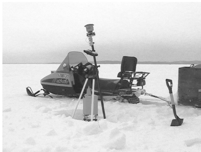
Figure 3. Picture taken during the 2004 survey. The gravimeter and the differential GPS system are shown as well as the snowmobile used for travel between stations.
